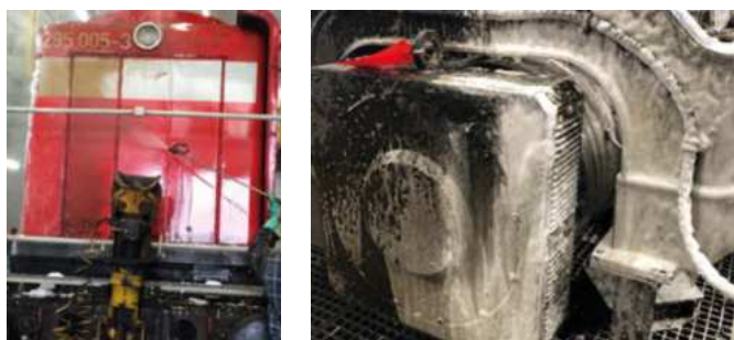
Applying cleaner with compressed-air foam lance
