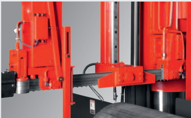
Additional blade guiding for trim cutting stabilization
