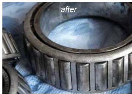
Cleaning with STAR US 6 in the ultrasonic cleaning device
