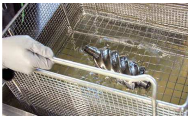
Cleaning a machine part in an ultrasonic bath
