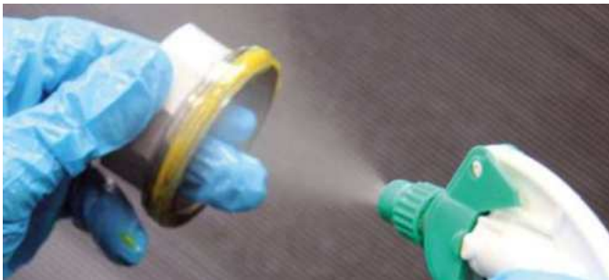
Removing sealant with GS 200
