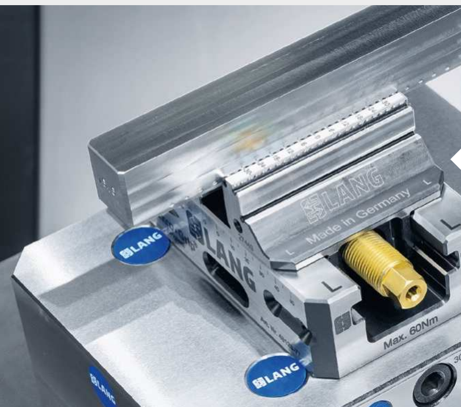
Material of the pre-stamped and clamped component: 1.2714 QT
