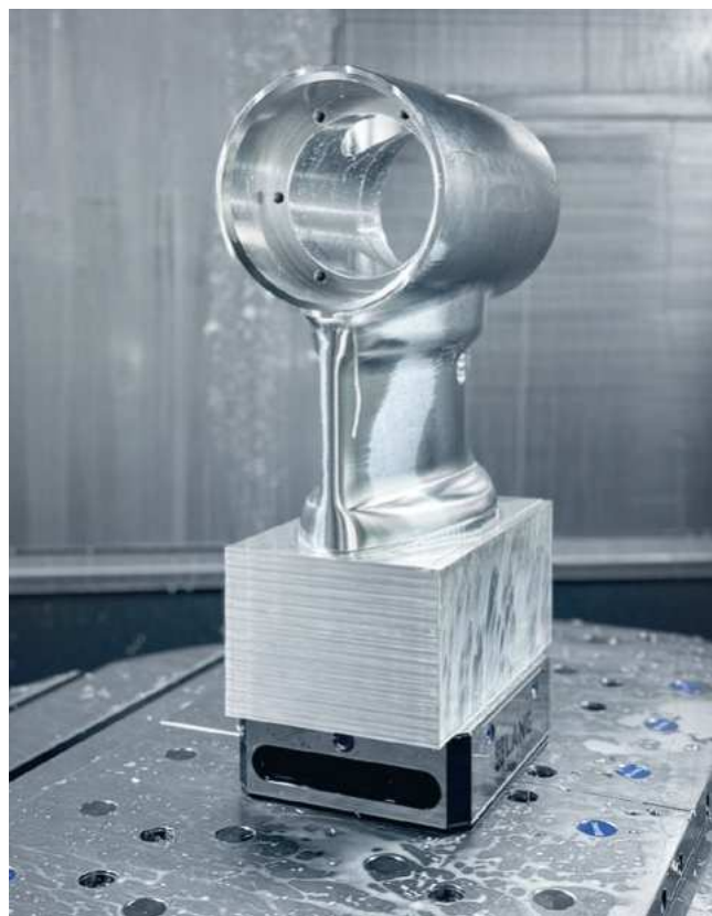
Direct clamping of a gearbox via four clamping studs with over 80% material removal.
